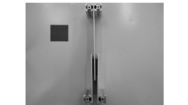
图 2 磁流变弹性体支撑结构 Fig. 2 Supporting structure based on MRE
