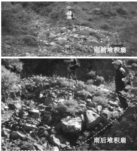
图 5 兴盛永沟堆积扇松散物源强降雨前后变动情况 Fig. 5 Comparison of the loose material volume for the Xingshengyong catchment before and after the heavy rainfall
