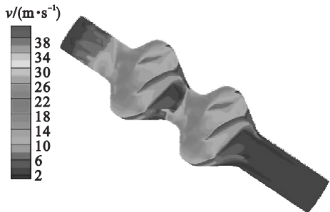
图 7 两级矿浆泵固液内流场绝对速度分布 Fig. 7 Absolute velocity distribution of two-stage slurry pump solid-liquid flow field
