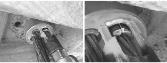
图 6 工作锚夹片拉出 Fig. 6 Clip is pulled out of the working anchor
