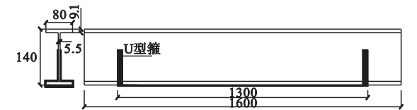
图 1 试件几何尺寸及加固方式 (mm) Fig. 1 Dimension of the specimens and strengthened method
