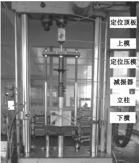
图 6 示功机实验台 Fig. 6 Testing bench of indicator machine
