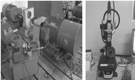
图2 多功能齿轮试验台与三维超景深显微系统 Fig. 2 Multi-function gear test rig and super depth of field three-dimensional microscope system
