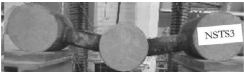
图 5 试件整体破坏形态 Fig. 5 Failure modes of the specimen
