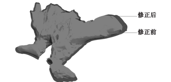
图 6 501-2 空区探测模型误差修正前后对比 Fig. 6 Comparison of error detection models before and after correction of 501-2
