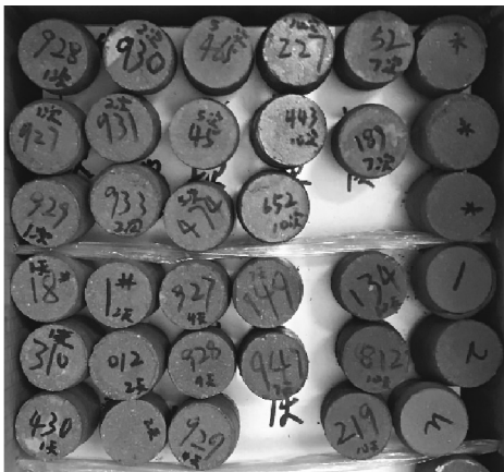
图 2 三轴压缩试样 Fig. 2 Samples after triaxial compression
