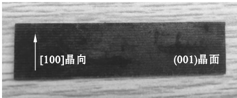
图 1 DD5 及其晶面和晶向 Fig. 1 DD5 and its crystal plane and orientation
