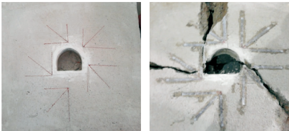
图 2 拱顶无空洞模型破坏 Fig. 2 The failure mode of tunnel model with no cavity at the crown
