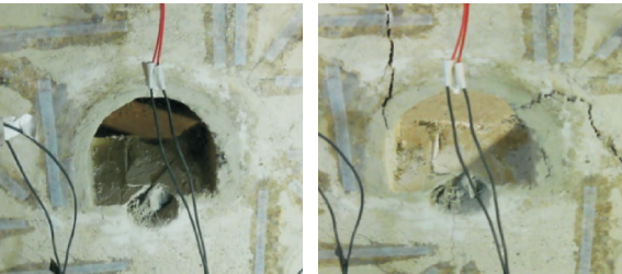
图 16 底板空洞模型破坏 Fig. 16 The failure mode of the tunnel model with a cavity at the floor
