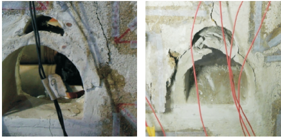
图 4 拱顶空洞模型破坏 Fig. 4 The failure mode of tunnel model with a cavity at the crown
