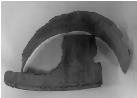
图 3 阴极电沉积产物 Fig. 3 Photographs of deposited product on cathode
