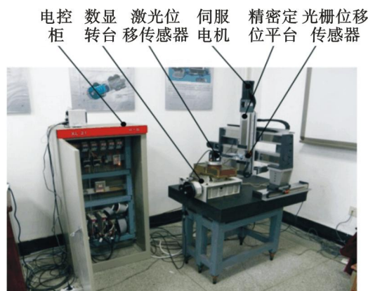
图5 三坐标测量机 Fig. 5 The three coordinate measuring machine
