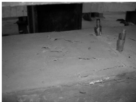
图 6 高温试验构件破坏图 Fig. 6 Typical failure mode of tested beams under high temperature
