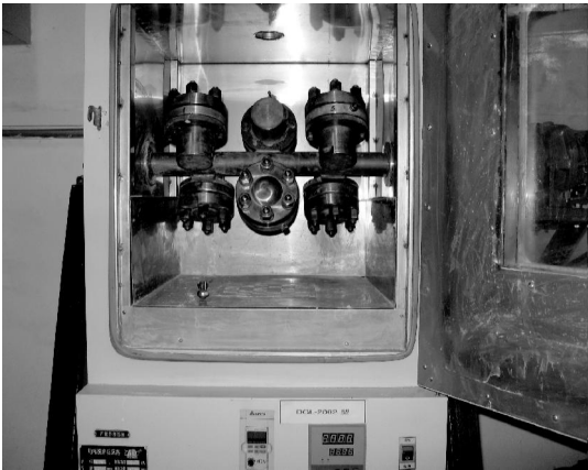
图 2 均相溶出反应釜 Fig. 2 Balanced ball milling reaction kettle
